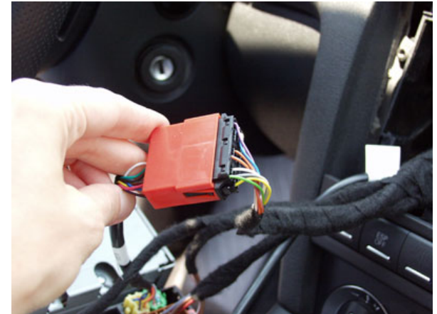
3. AUDES adapter connected to Factory Black Connector
