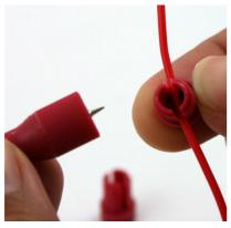
Insert wire, (referred as "HOT") that is to be tapped - the one that comes out of your stereo main harness, down the gap in the cap as far as it will go.
