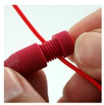
This is when the tap is started onto the threads of the larger cap. Keep the posi-tap straight so the pin is centered on the wire when it contacts the wire.
