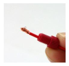
Unscrew the smaller cap and insert striped wire end through it, making sure all strand get through. Then fold wires over to one side.
