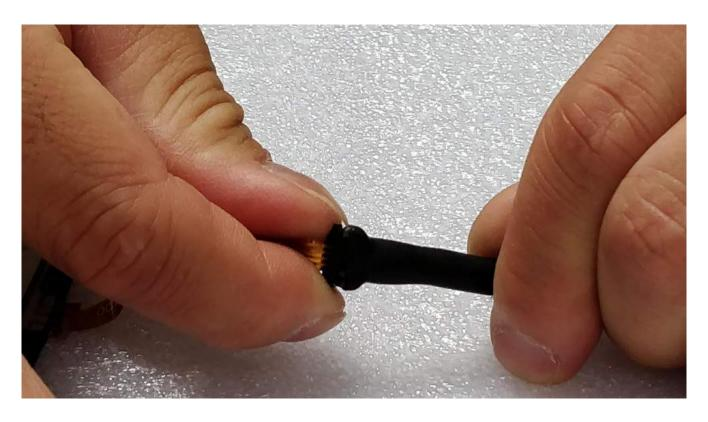
Carefully press locking connector towards the middle and down to the V-TOUCH cable, to secure the pins on the ribbon cable in place.
