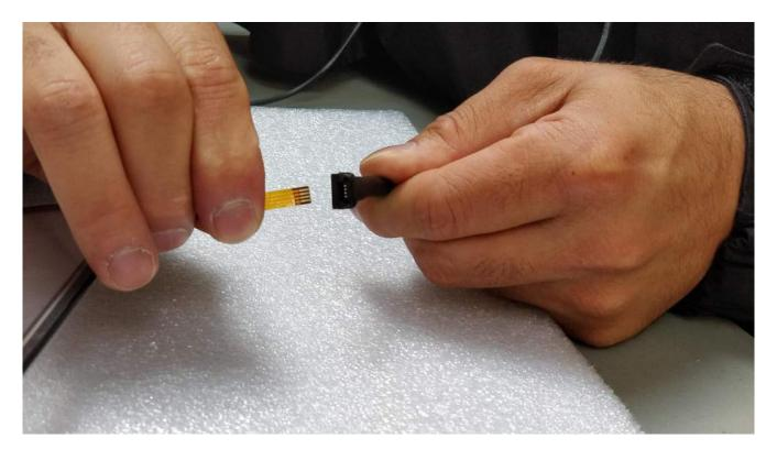
Connect ribbon cable to the V-TOUCH cable. The exposed pins on the ribbon cable should face up. The pins on the V-TOUCH cable should face up.
