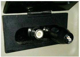
3. Leave it connected at all times with no wires connected to it and this should resolve poor sound issue with GROM audio playback.
