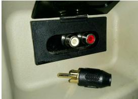
1. Locate RCA cable scrape or one you do not care about and cut wire off end of it. We will only use the RCA connector end of it.
