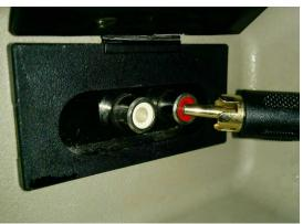
2. Plug the RCA connector into the RED side o the factory Auxiliary port
