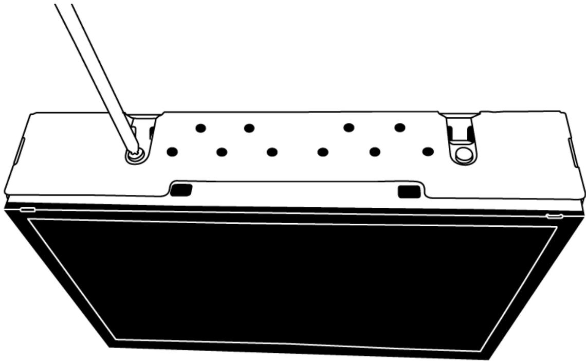
Remove 2 Phillips screws from top of LCD enclosure
