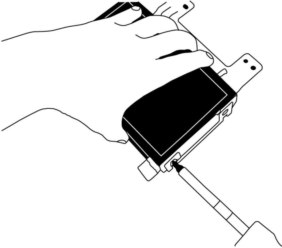
Screw the metal bracket back to the LCD assembly
