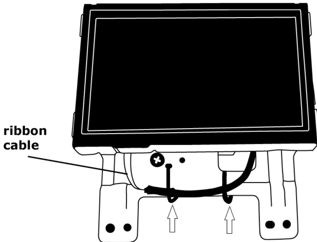
Carefully route the V-TOUCH cable assembly through the cut-out in the metal bracket to the back side of LCD screen assembly.
