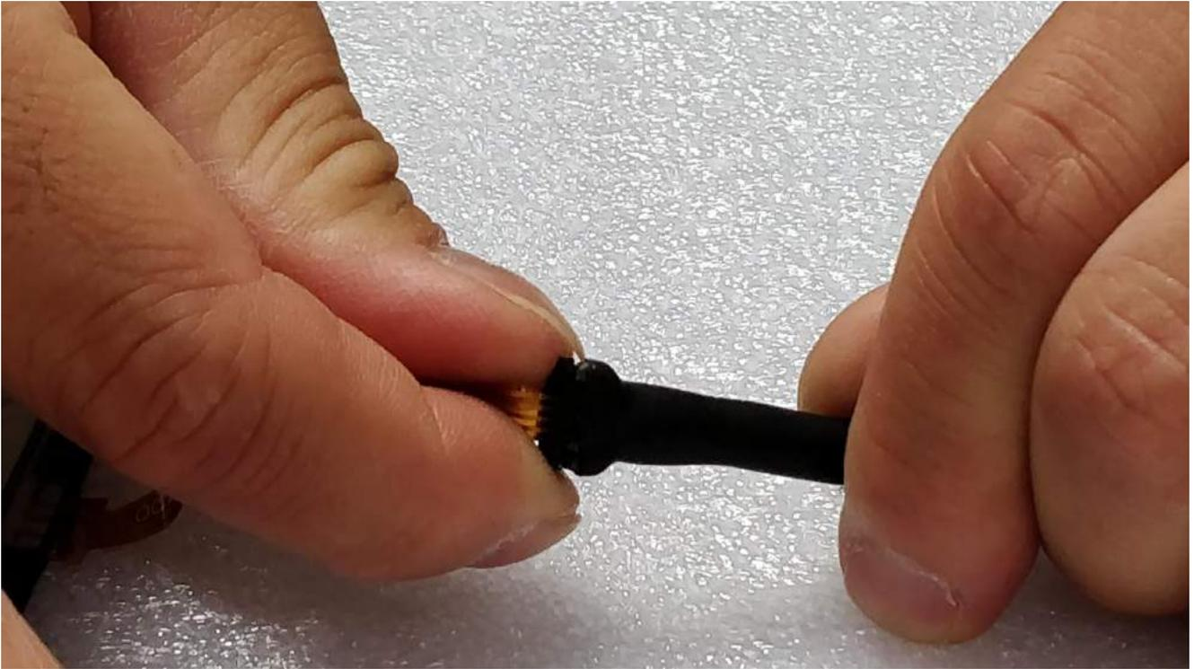
Carefully press locking connector towards the middle and down to the V-TOUCH cable, to secure the pins on the ribbon cable in place.
