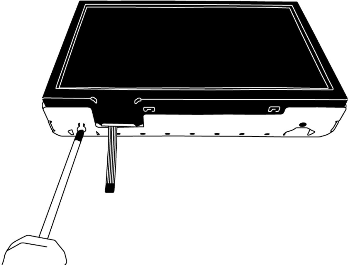
Reinstall the 4 Phillips screws, 2 on top 2 on bottom
