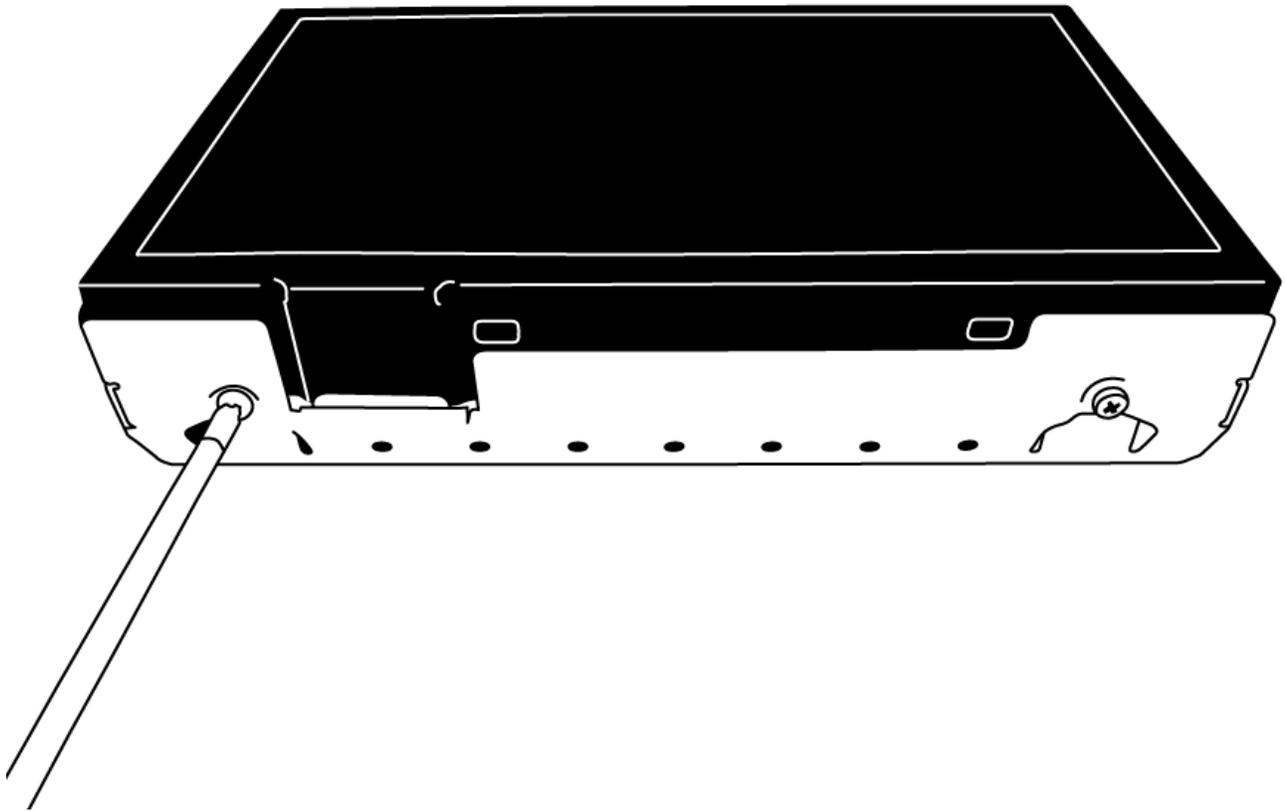
Remove 2 Phillips screws from bottom of LCD enclosure
