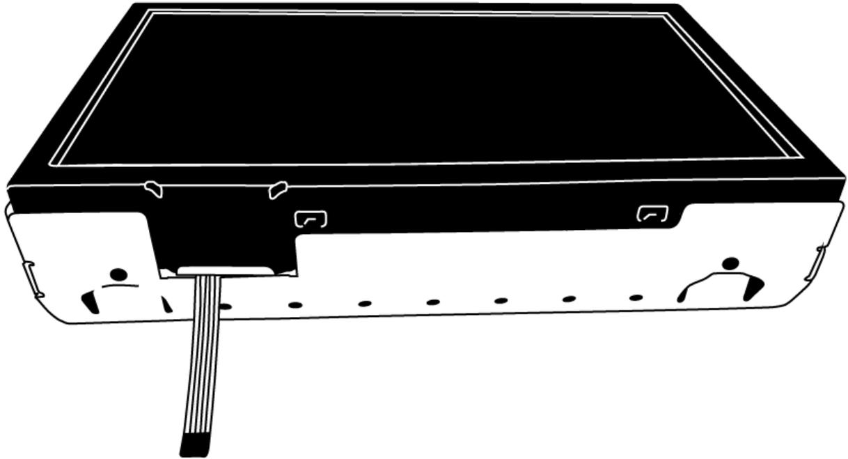
Make sure the 4pin ribbon cable from the touchscreen panel comes through the enclosure gap
