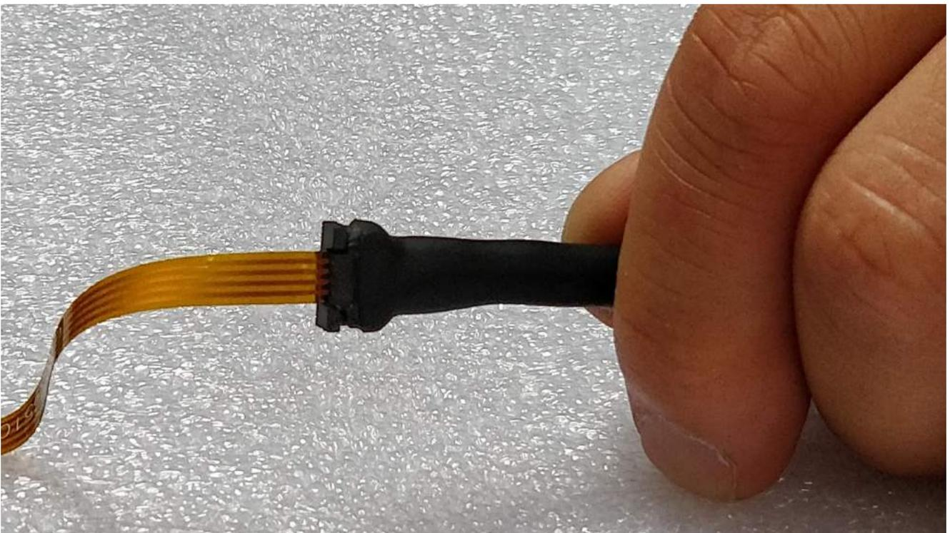
Connect the other end of V-TOUCH cable to the TSB1 controller board, as shown below.
