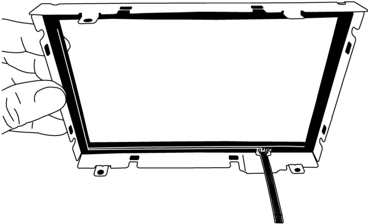
How the new touchscreen panel should look in the front bezel, note that the 4pin ribbon cable sits within the notch on the bezel.
