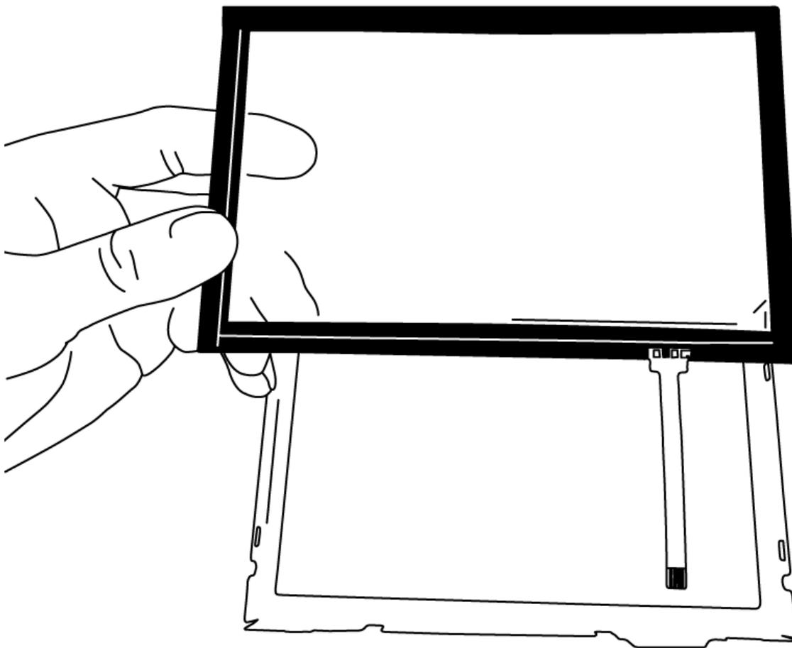
Remove protective plastic from the front side of the supplied touchscreen panel, and carefully install the supplied touchscreen panel in place of the now removed factory clear screen cover.
