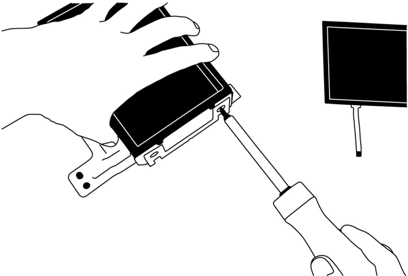
2. Remove 4 Phillips screws from both sides of vehicle's LCD screen assembly, and remove LCD assembly from the metal bracket.
