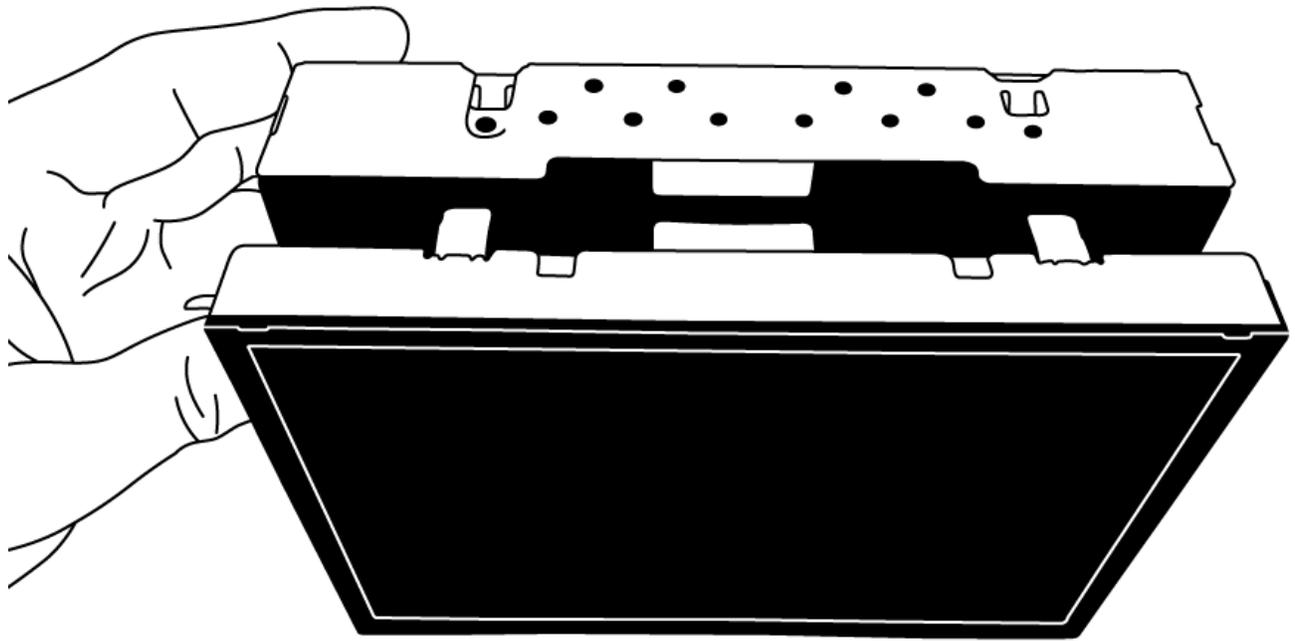
Now remove the back metal cover from the LCD assembly
