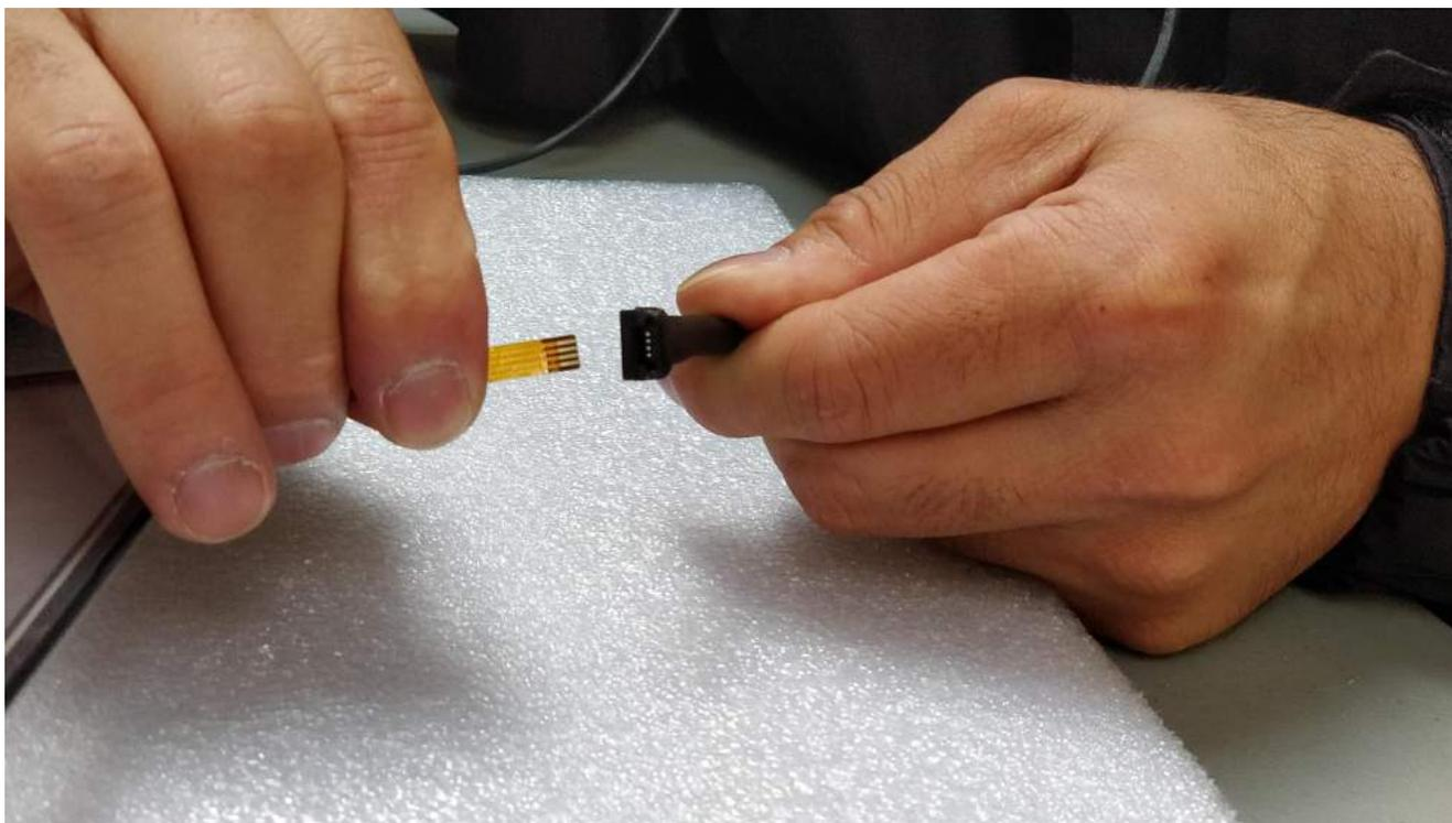
Connect ribbon cable to the V-TOUCH cable. The exposed pins on the ribbon cable should face up. The pins on the V-TOUCH cable should face up.
