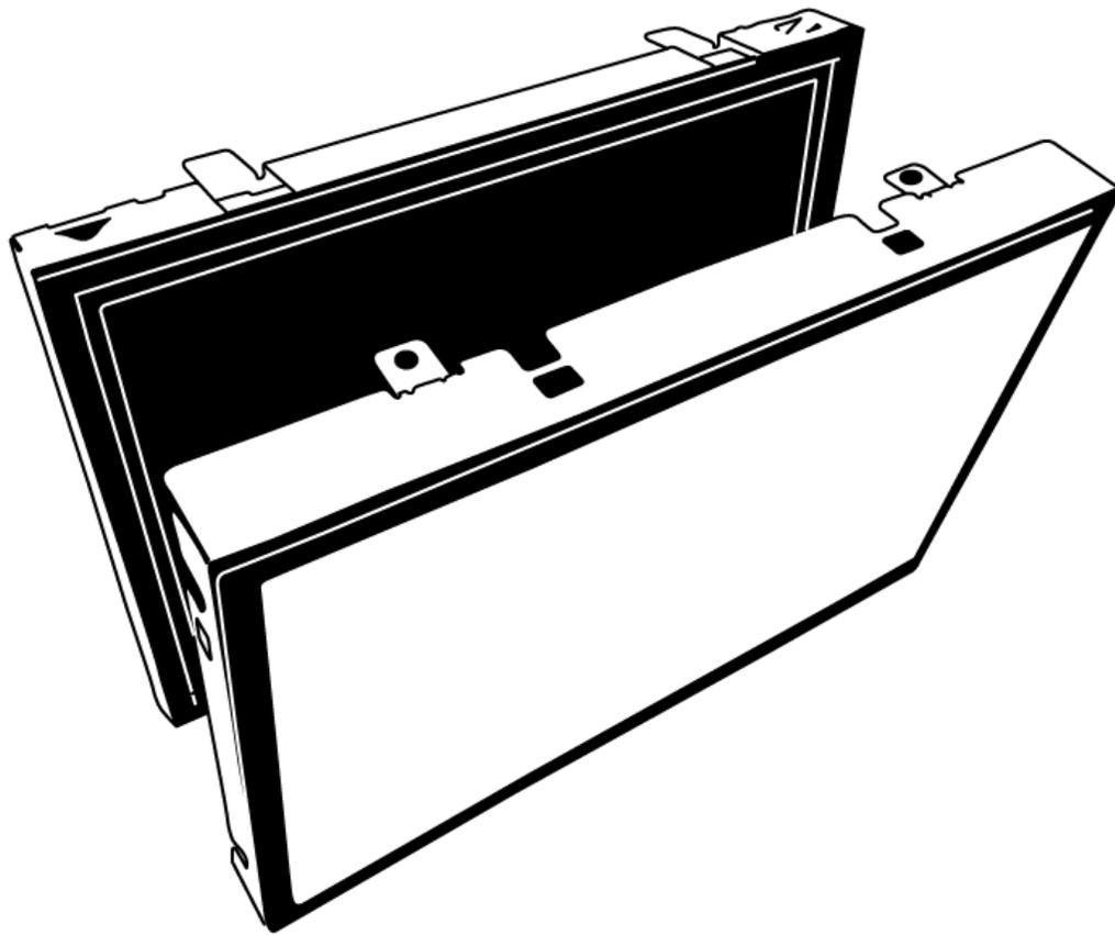
Using the awl tool, remove the front bezel from the LCD assembly
